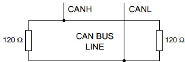
Each end of the CAN bus is terminated with 120Ω resistors in compliance with the standard to minimize signal reflections on the bus. You may need to place a 120Ω terminating resistor between CAN-L and CAN-H
