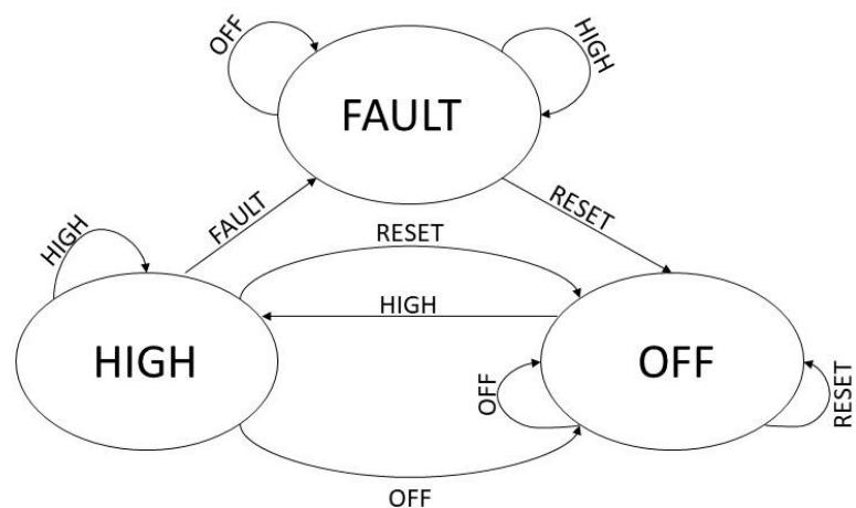
The output pin of each output circuit can be in one of the 3 following states:
