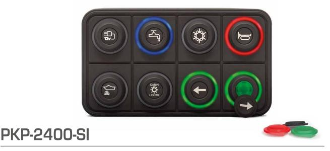
**PKP-2400-SI** is a compact keypad based on CAN protocol. It comes equipped with eight keys with interchangeable 15 mm inserts. The keypad is water and dust resistant, and can be installed both inside and outside the cockpit. RGB LED lights and the ease with which icons can be switched in and out make it possible for the user to customize each key in a wide range of variations.
