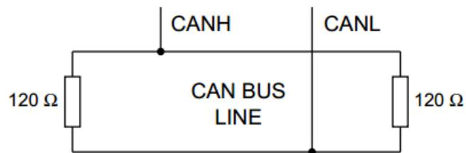
Each end of the CAN bus is terminated with  $120\Omega$  resistors in compliance with the standard to minimize signal reflections on the bus. You may need to place a  $120\Omega$  resistor between CAN-L and CAN-H.
