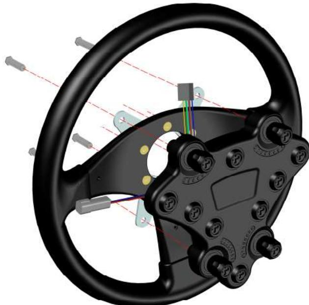
3: plug the connectors to complete the installation.
