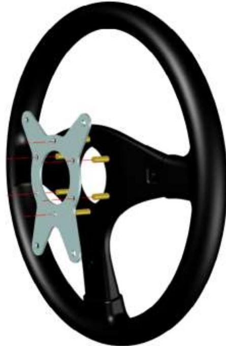
2: assemble the Racepad to the steering wheel by fastening the M5 screws along the four holes of the metal plate and the backshell. Bend the wires to the preferred side to simplify the installation on the steering wheel.
